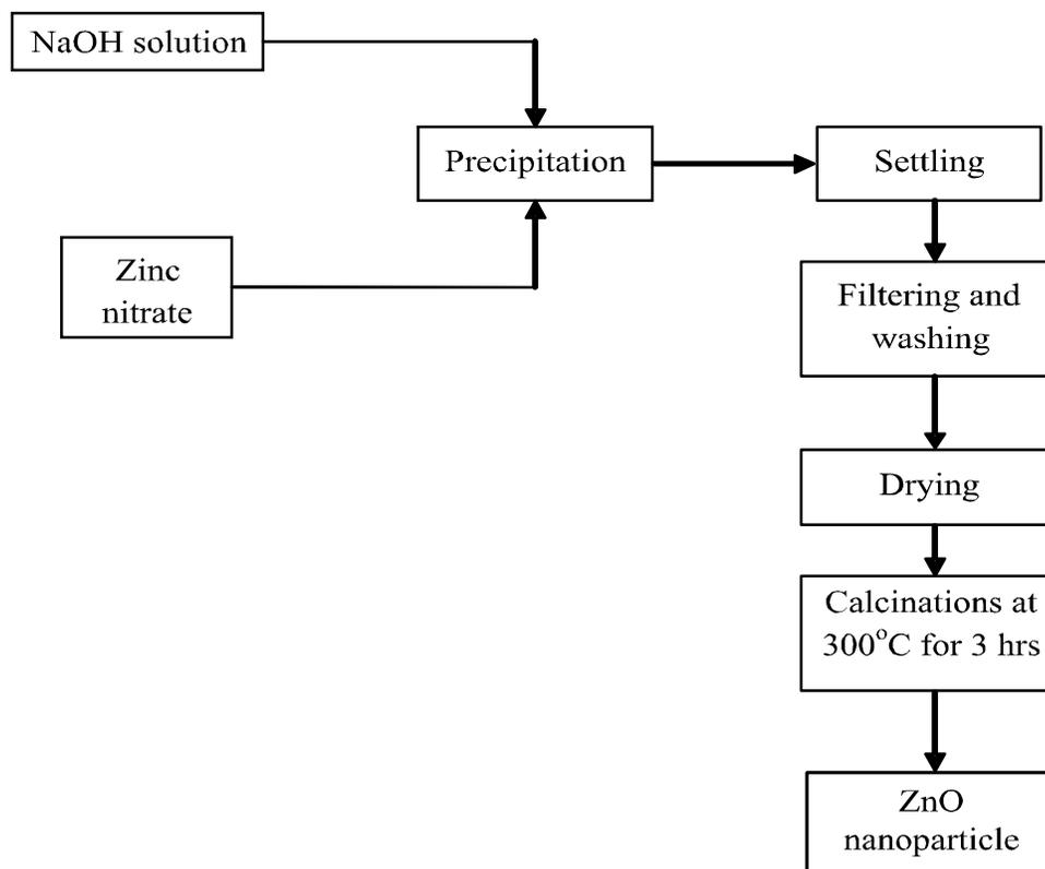
**Fig. 1: Schematic of sample preparation using precipitation method**
