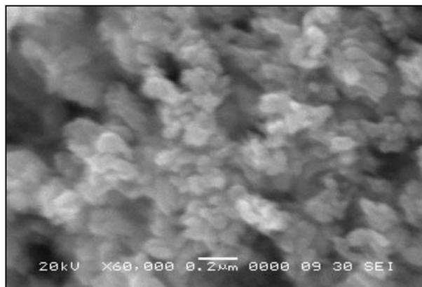
**Fig. 3: SEM image of ZnO nanoparticles**
