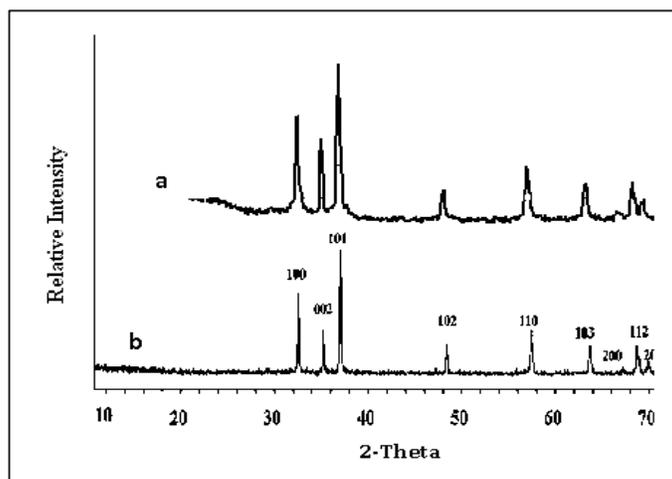
**Fig. 2: The XRD pattern (a) prepared ZnO and (b) commercial ZnO**
