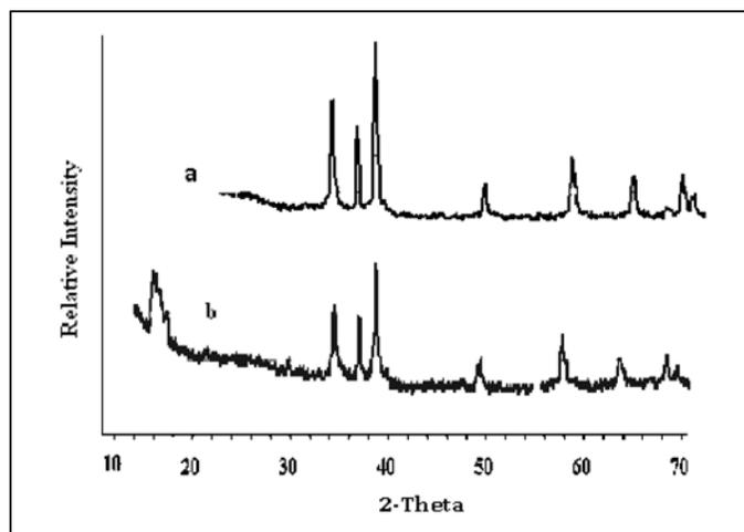
**Fig. 5: XRD pattern for (a) ZnO nanoparticles and (b) 50% ZnO-Bentonite nanocomposite**
