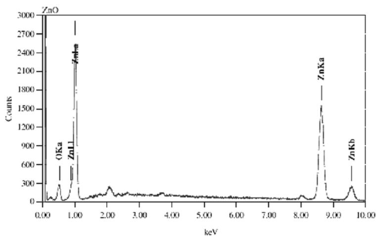
**Fig. 4: EDX analysis of ZnO nanoparticles**
