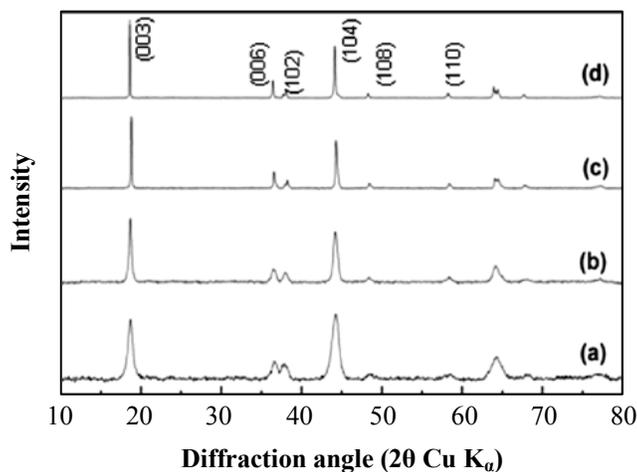
**Fig. 3: X-ray diffraction patterns of bare  $\text{LiNi}_{0.3}\text{Mn}_{0.3}\text{Co}_{0.3}\text{O}_2$  and Zn doped  $\text{LiNi}_{0.3}\text{Mn}_{0.3}\text{Co}_{0.3}\text{O}_2$  (a)  $x = 0.00$  at  $800^\circ\text{C}$  (b)  $x = 0.00$  at  $1000^\circ\text{C}$  (c)  $x = 0.01$  at  $1000^\circ\text{C}$  (d)  $x = 0.02$  at  $1000^\circ\text{C}$**
