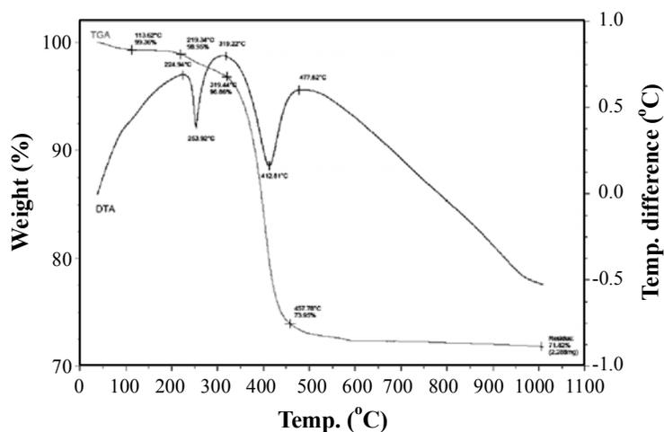
**Fig. 1: TG curve for Bare  $\text{LiNi}_{0.3}\text{Mn}_{0.3}\text{Co}_{0.3}\text{O}_2$**
