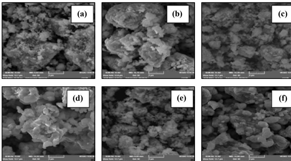
**Fig. 4: SEM images of bare Zn doped  $\text{LiNi}_{0.4}\text{Mn}_{0.3}\text{Co}_{0.3}\text{O}_2$  samples (a)  $x = 0.00$  at  $800^\circ\text{C}$ , (b)  $x = 0.00$  at  $1000^\circ\text{C}$ , (c)  $x = 0.01$  at  $800^\circ\text{C}$ , (d)  $x = 0.01$  at  $1000^\circ\text{C}$ , (e)  $x = 0.02$  at  $800^\circ\text{C}$  & (f)  $x = 0.02$  at  $1000^\circ\text{C}$**
