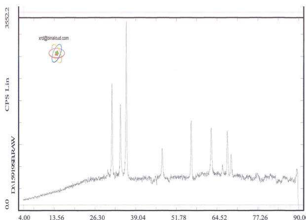
Figure 3 : XRD pattern of  $Pb_2(SO_4)O$  produced by calcinations of  $[Pb(bpy)(NCS)_2]_n$
