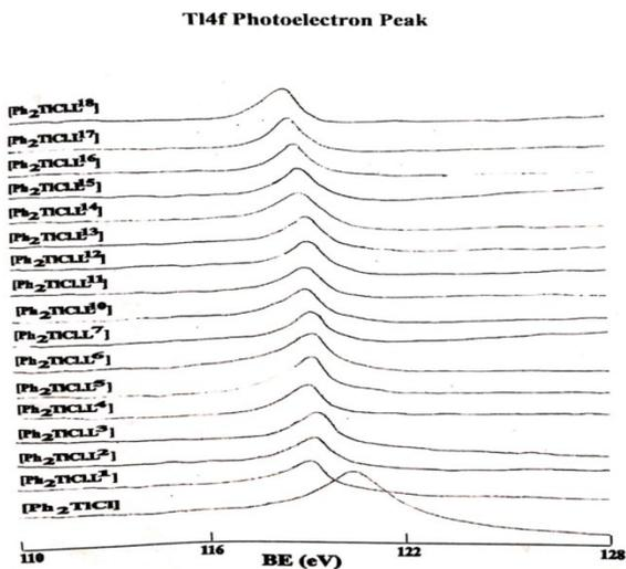
FIG. 1. T14f binding energies (ev)  $(Ph_2TiCl)$  and  $(Ph_2TiClL)$  complexes.
