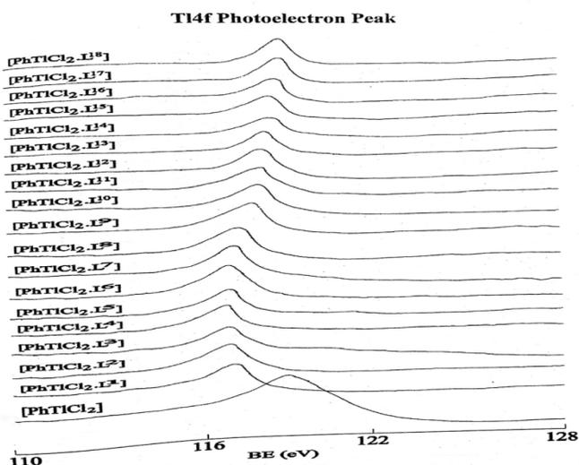
FIG. 2. T14f binding energies (ev)  $(PhTiCl_2)$  and  $(PhTiCl_2L)$  complexes.
