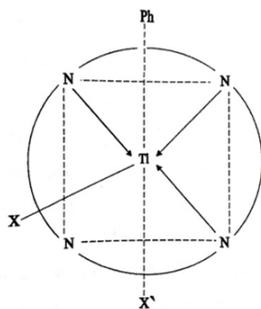
FIG. 6. Octahedral Geometry of (Ph<sub>2</sub>TiCl.L) complexes, Where In (Ph<sub>2</sub>TiCl.L)= X=Cl; X<sub>1</sub>= Ph, In (PhTiCl<sub>2</sub>.L)= X= Cl; X<sub>1</sub>=Cl.
