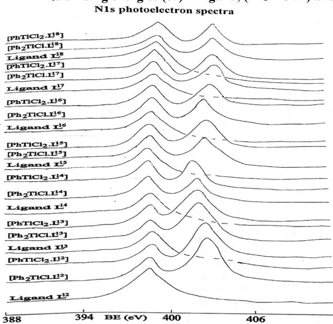
FIG. 5. N1s binding energies (ev) in ligand, (Ph<sub>2</sub>TiCl.L) and (PhTiCl<sub>2</sub>.L) complexes.
