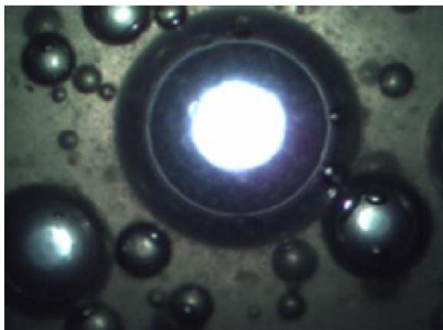
**Figure 1: Microstructure of fuzzy ball working fluid under 1000 times microscope**
