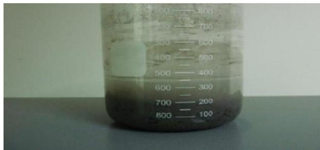
**Figure 2 : Fuzzy ball bionic drilling fluid after flocculation**
