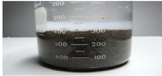
**Figure 3 : Fuzzy ball bionic drilling fluid after gel-breaking** after gel-breaking can satisfy the secondary standard of “GB8978-96 National Sewage Discharge Standard”, which can be discharged directly.
