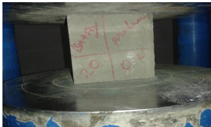
FIG. 1. Compressive strength Test of FA and QD Cube.
