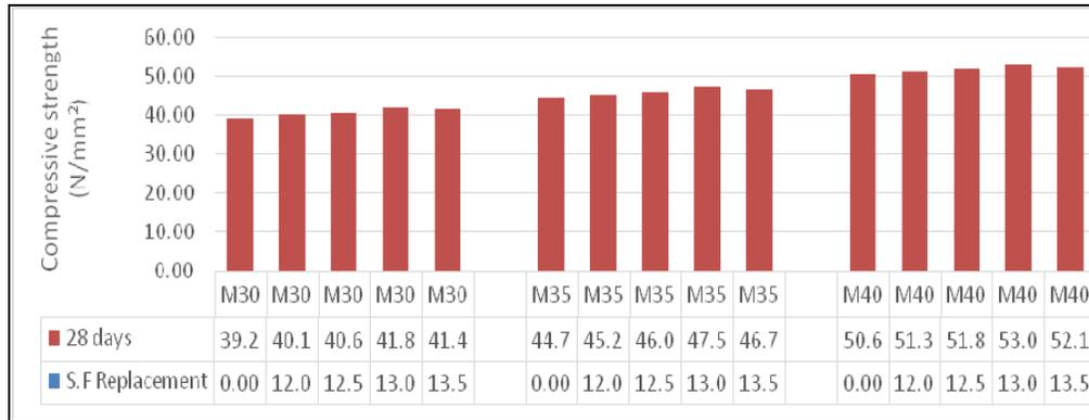
**Fig. 2: 28 Days cube compressive strength (N/mm<sup>2</sup>)**
