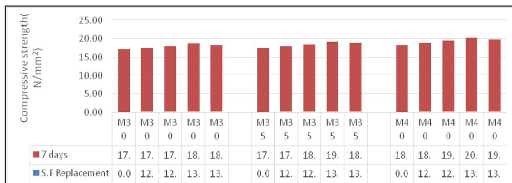
Fig. 1: 7 Days cube compressive strength (N/mm<sup>2</sup>)
