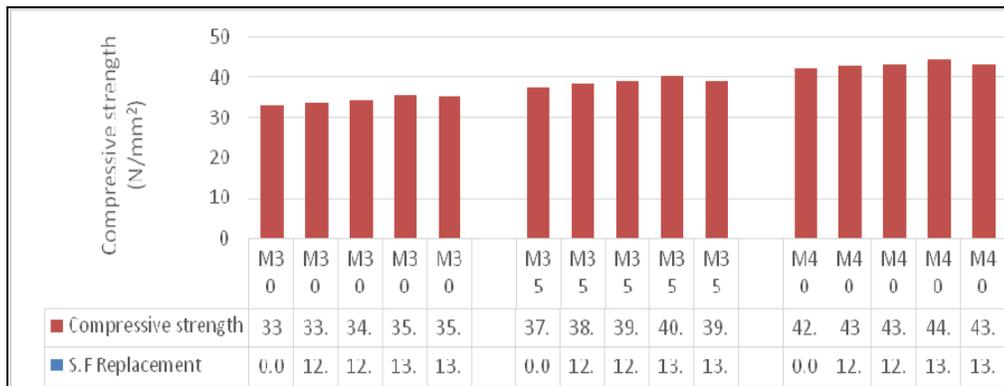
**Fig. 3: 28 Days cylinder compressive strength (N/mm<sup>2</sup>)**
