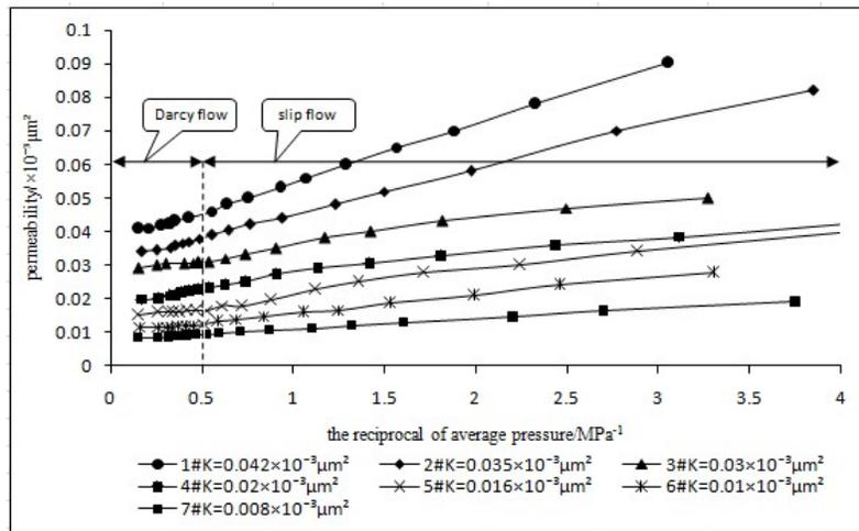
Figure 4 : Klinkenberg curve of rock samples with permeability less than  $0.05 \times 10^{-3} \mu\text{m}^2$
