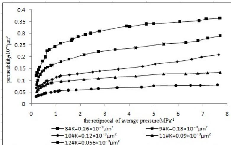
Figure 5 : Klinkenberg curve of rock samples with permeability more than  $0.05 \times 10^{-3} \mu\text{m}^2$
