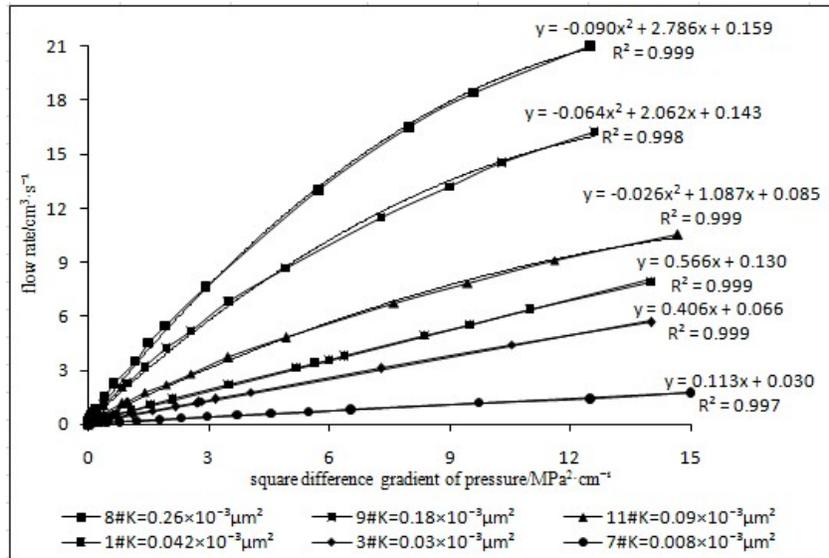
Figure 7 : Relation curve of flow rate and square difference gradient of pressure
