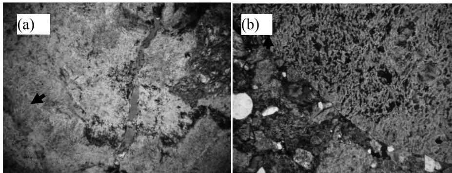
Figure 2 : Core casting thin section of igneous gas reservoir
