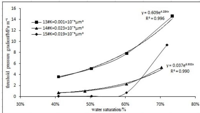
Figure 8 : Relation curve of threshold pressure gradient and water saturation
