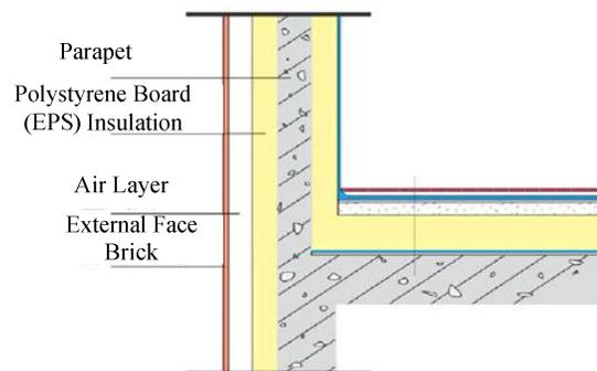
**Figure 2 : Thermal insulation of closed roof**
