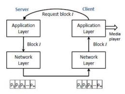
Figure 1: The structure of network coding layer
