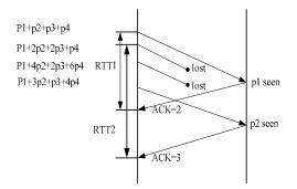
Figure 6: ACK acknowledgement mechanisms
