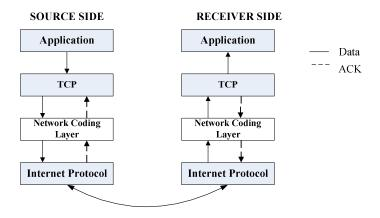
Figure 4 : Structural diagram of network coding level
