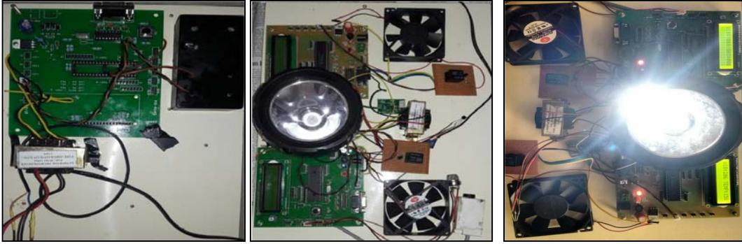
**Fig. 4: Receiver, transmitter and output section for Li-fi technology**
