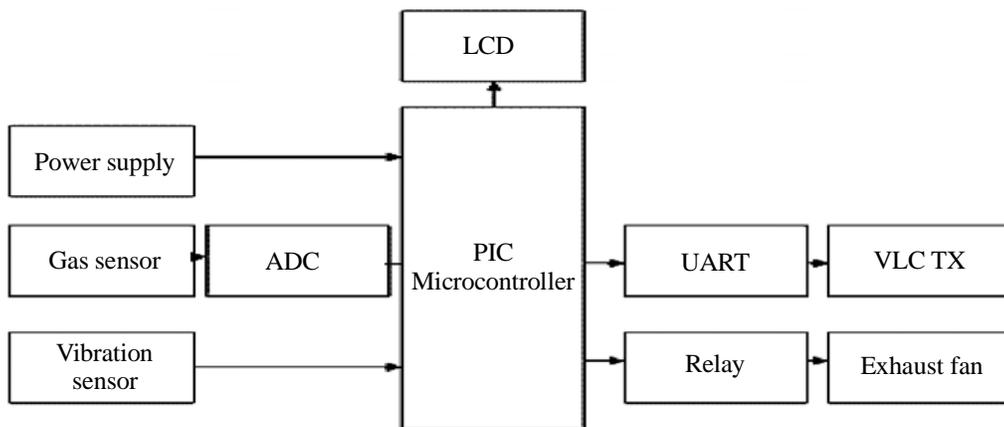
**Fig. 2: Block diagram of Node 2**
