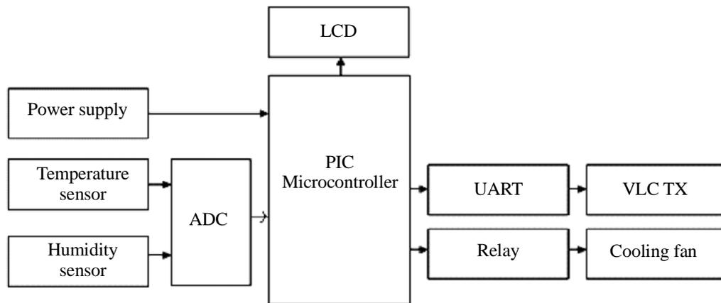
**Fig. 1: Block diagram of Node 1**
