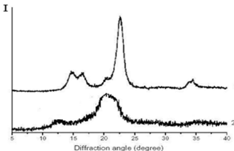
Figure 1 : X-ray diffractograms of acid-hydrolyzed cotton (1) and regenerated cellulose (2)
