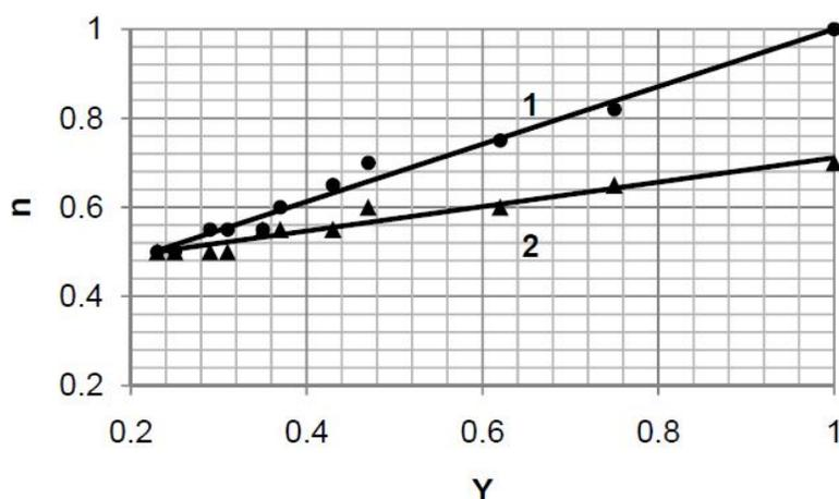
Figure 8 : Dependence of coefficient (n) on the content of amorphous domains of cellulose (Y) for undried (1) and dried (2) samples
