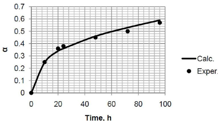
Figure 7 : Calculated and experimental kinetics of enzymatic hydrolysis of dried cotton linter (CL)
