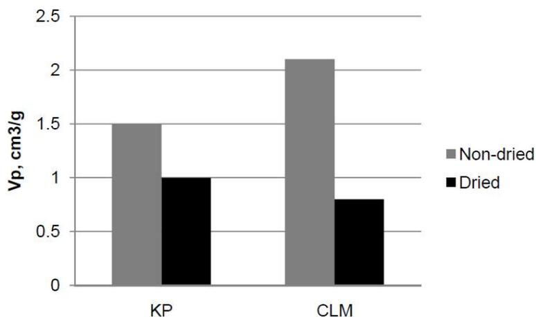
Figure 2 : Pore volume for not dried and dried cellulose samples: kraft pulp (KP) and mercerized cotton linter (CLM)
