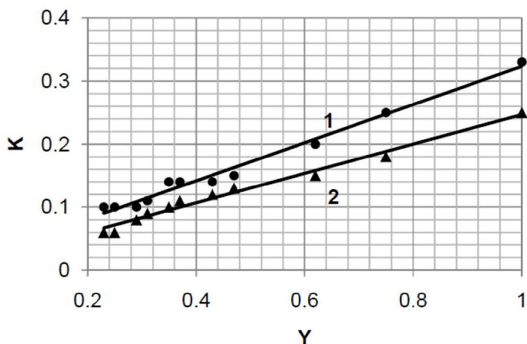
Figure 9 : Dependence of effective rate constant (K) on the content of amorphous domains of cellulose (Y) for undried (1) and dried (2) samples
