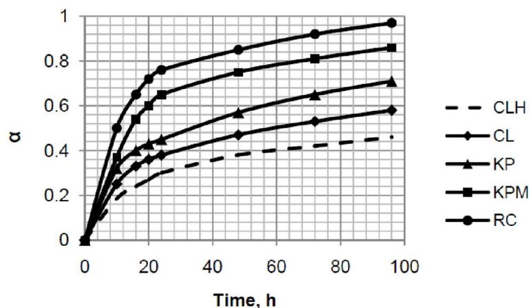
Figure 4 : Kinetics of the enzymatic hydrolysis of dried cellulose samples
