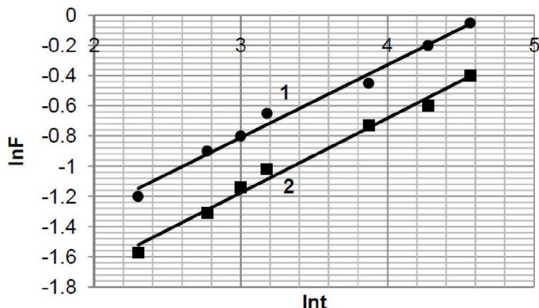
Figure 5 : Linearized kinetics of the enzymatic hydrolysis of undried (1) and dried (2) samples of hydrolyzed cotton linter (CLH)
