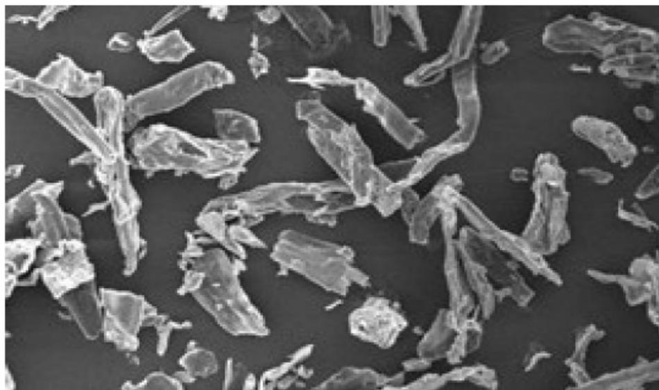
Figure 4 : Micro-photograph of microcrystalline cellulose (magnification 300 x)
