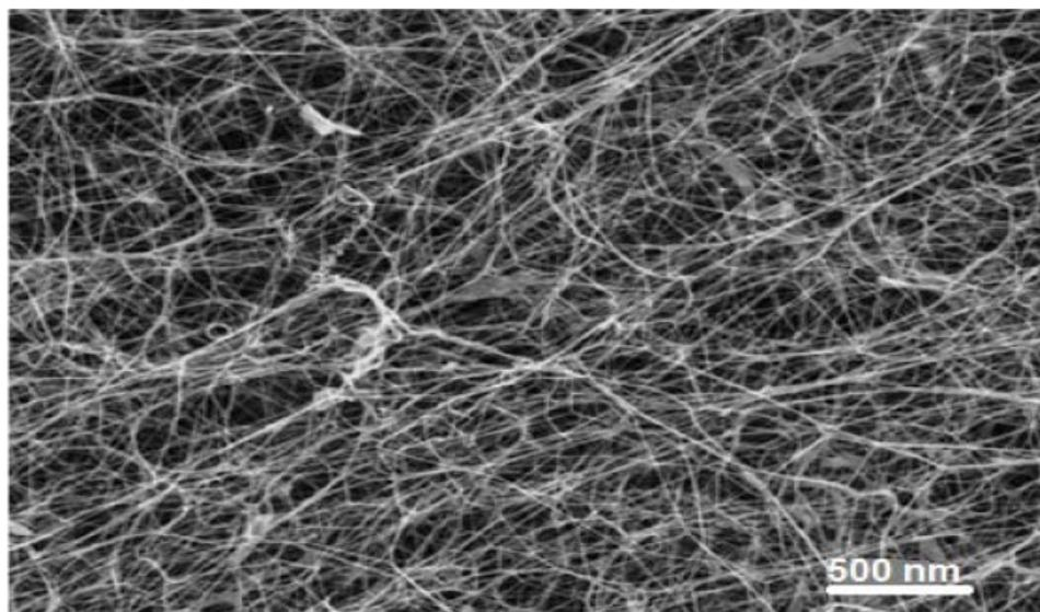
Figure 3 : SEM-image of bacterial nanocellulose
