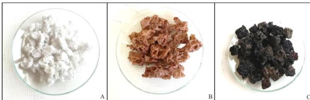
FIG. 4. Images of the nano porous silica beds in the three steps including: (A) before activation with Piranha solution, (B) after activation with Piranha solution and depositing of Lewis-Acid ( \text{FeCl}_3 ) or Subproduct-A, (C) after desulfurization process.
