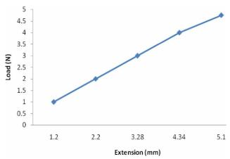
Figure 2 : Flexural property of TRHDPE plastic showing the Loading versus bending extension
