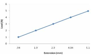
Figure 3 : Flexural property of VRHDPE plastic showing the loading versus bending extension
