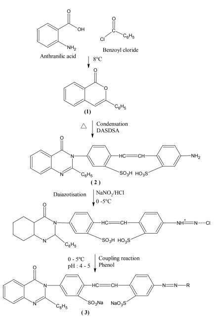
Where R = Phenol, o-Cresol, m-Cresol, p-Cresol, o-Cl-Phenol, m-Cl-Phenol, I-Naphthol, 2-Naphthol, Salicyclic acid, Resorcinol, H-acid, J-acid, R-acid and Gama acid for  $D_{g1}$  to  $D_{105}$  respectively
