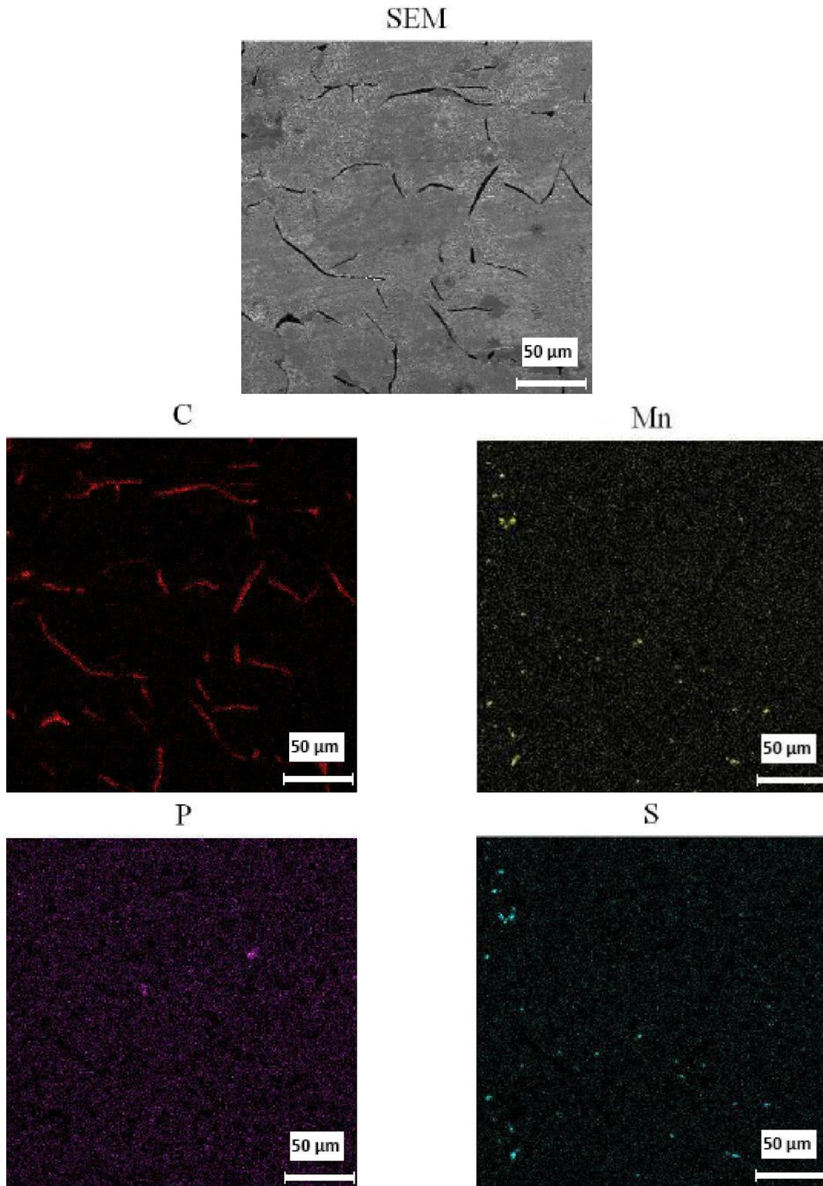
Figure 2 : SEM micrograph together with X-ray maps of semi-solid casting( $f_s=0.05$ ).
