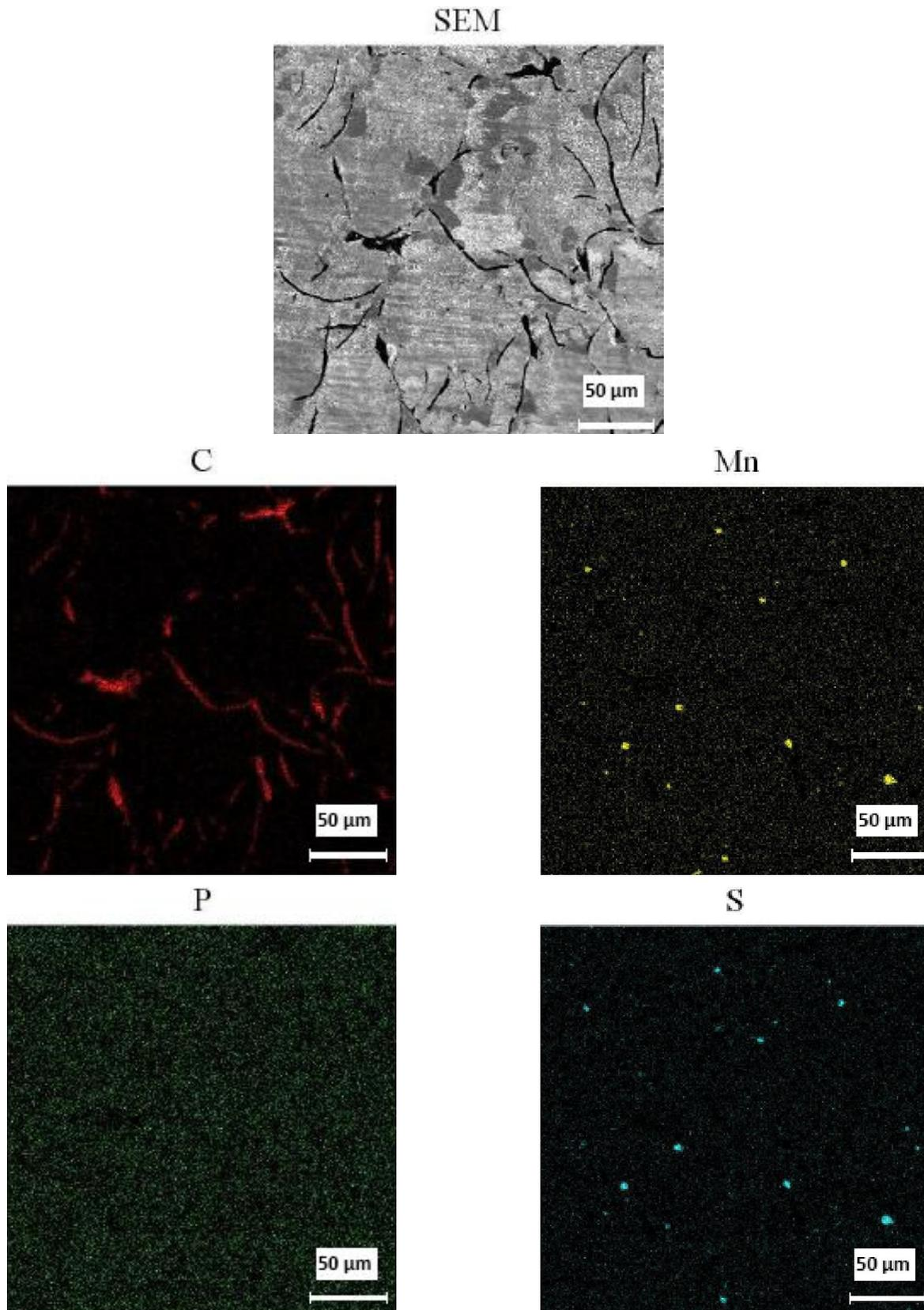
Figure 1 : SEM micrograph together with X-ray maps of ordinary casting.
