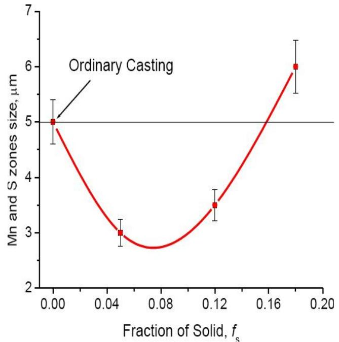
Figure 5 : Effect of fraction of Solid on Mn and S zones size.
