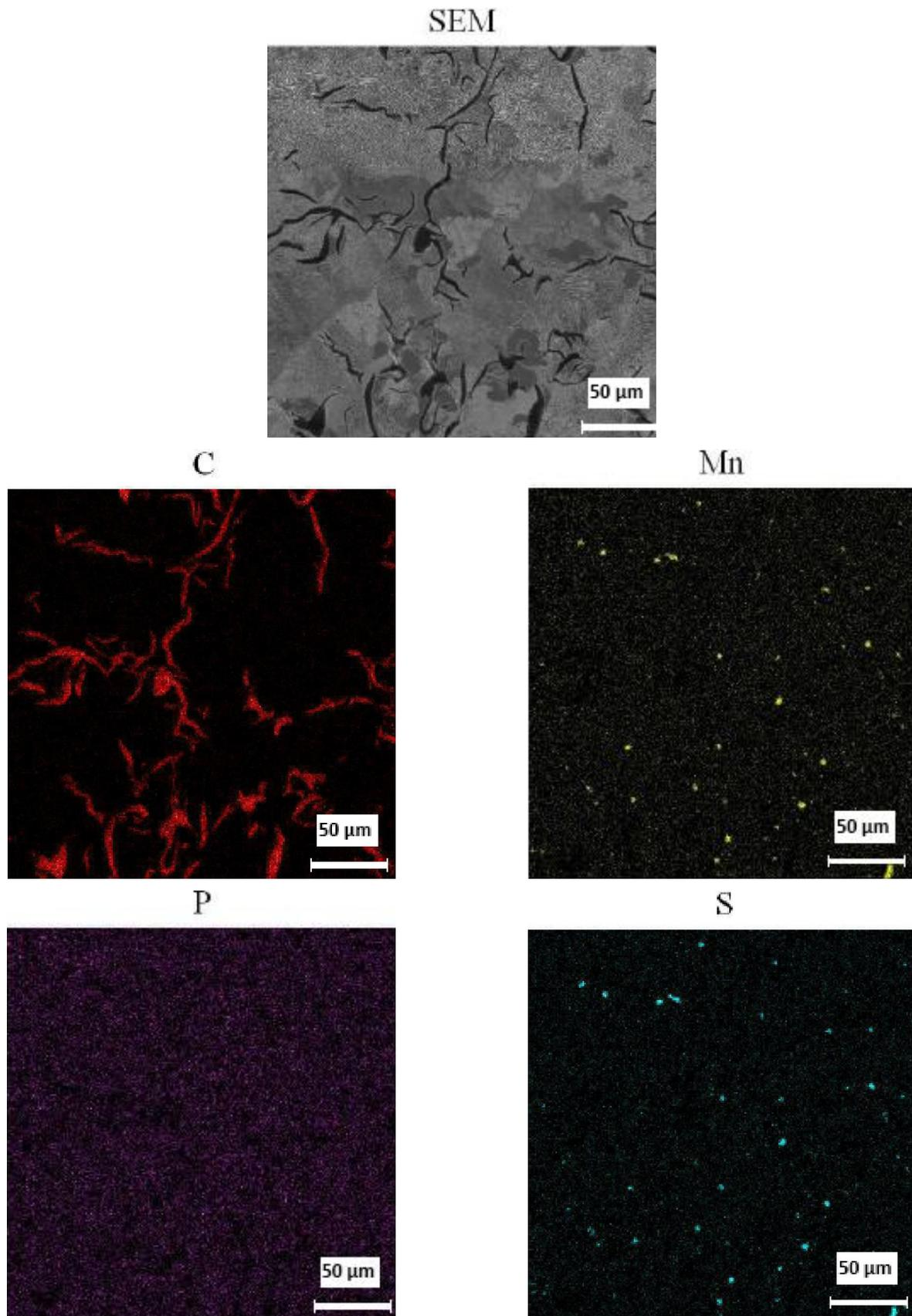
Figure 3 : SEM micrograph together with X-ray maps of semi-solid casting ( $f_s=0.12$ ).
