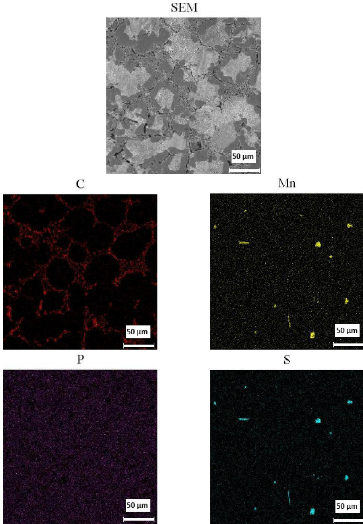
Figure 4 : SEM micrograph together with X-ray maps of semi-solid casting ( $f_s=0.18$ ).
