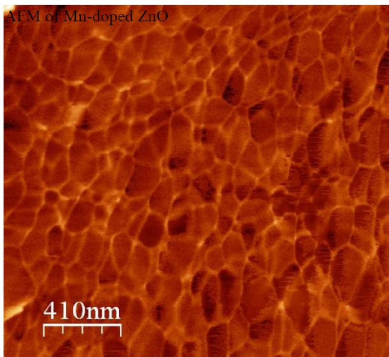
Figure 4 : AFM image of ZnO nanoparticle film.
