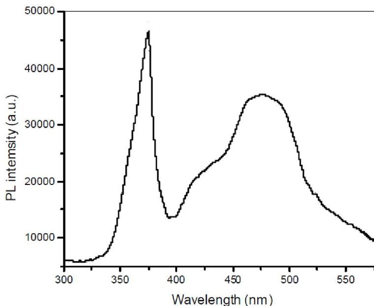
Figure 6 : PL spectrum of ZnO nanoparticle thin film.
