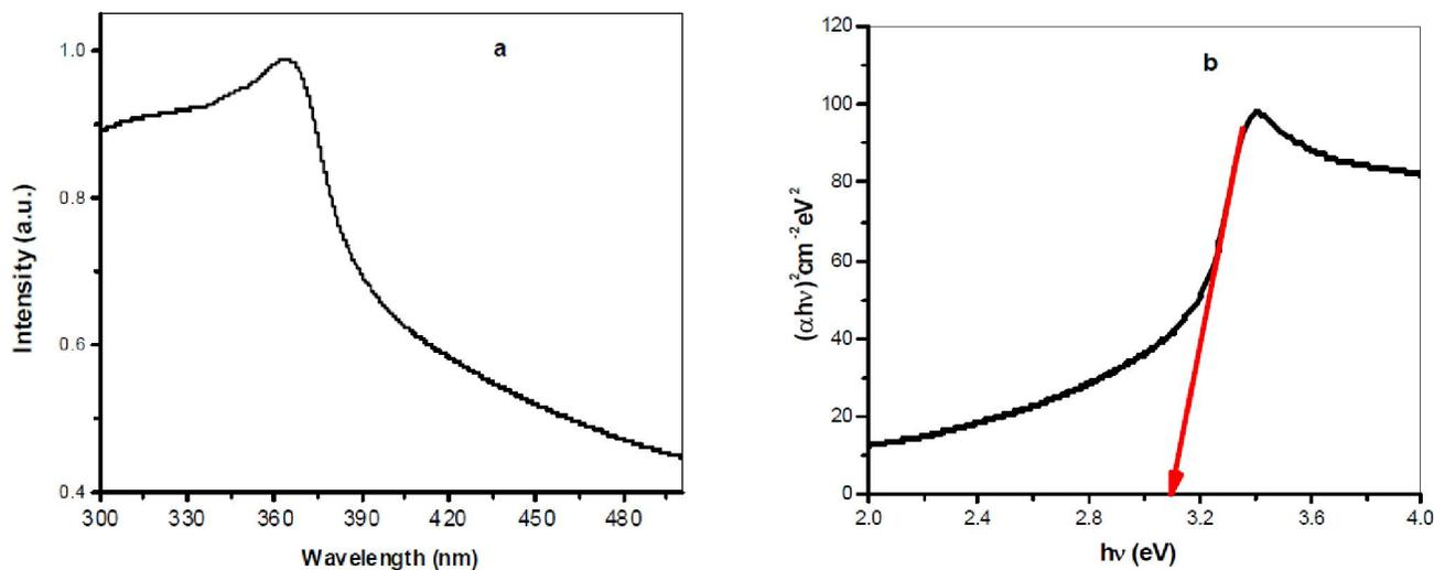
Figure 5 (a,b) : UV-vis spectra and optical band gap spectra of ZnO nanoparticle thin film.
