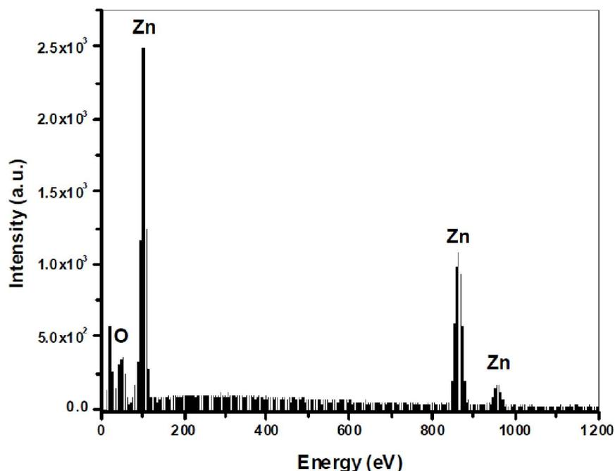
Figure 3 : EADX spectrum of the ZnO nanoparticle thin films.
