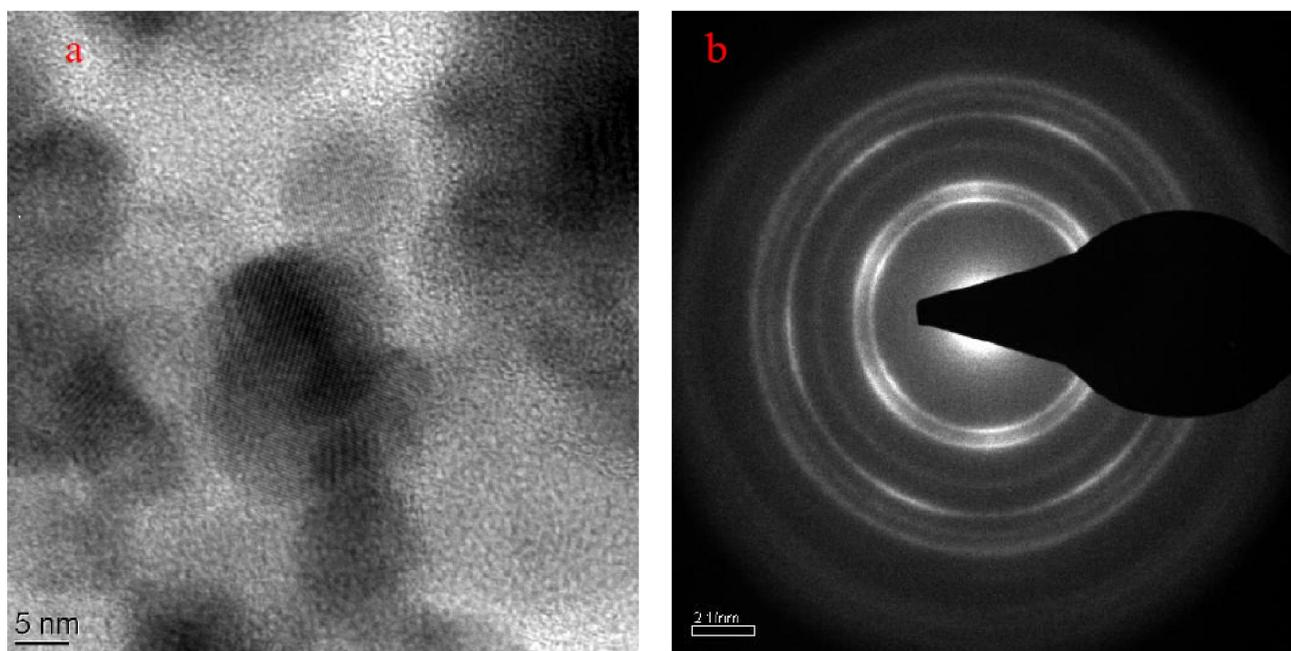
Figure 2(a,b) : TEM micrograph and selected area electron diffraction (SAED) pattern and of ZnO nanoparticle thin film
