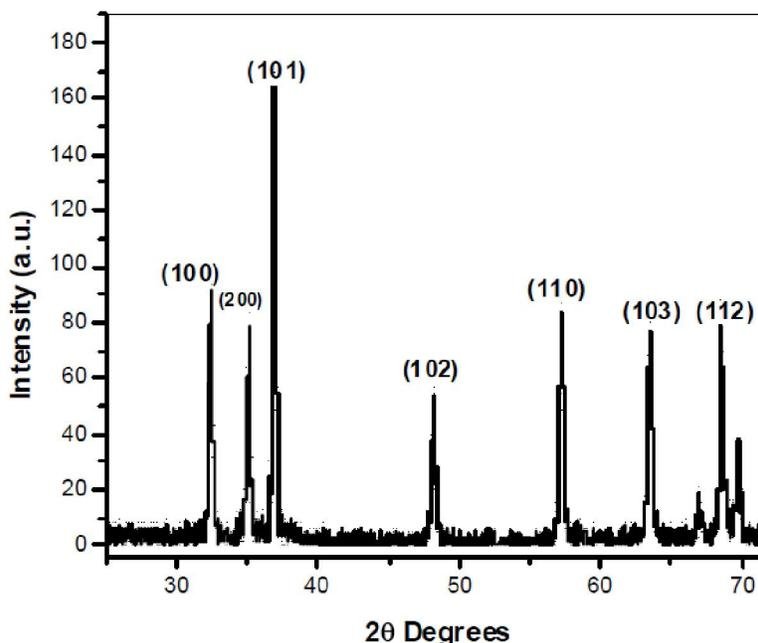
Figure 1 : XRD diffraction pattern of the ZnO nanoparticle thin films
