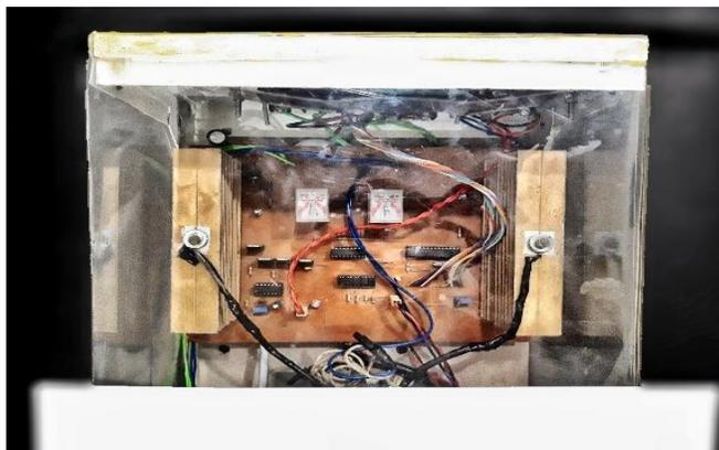
**FIG. 2.2 Microcontroller connections (smart solar inverter)**
