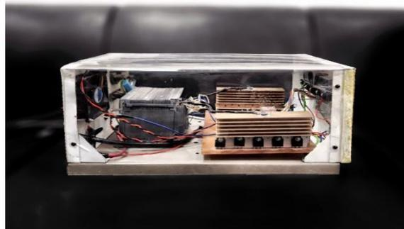
**FIG. 2 Hardware model (smart solar inverter).**
