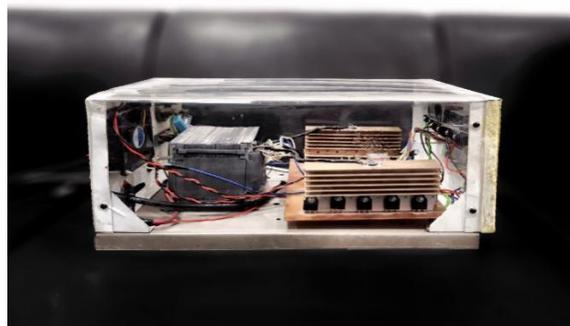
**FIG. 2 Hardware model (smart solar inverter).**
