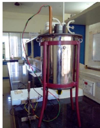
Figure 1: ENZextractor: Schematic and Desktop 3L Scale extractor
