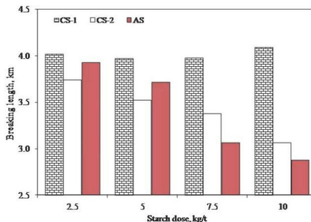
Figure 3 : Effect of starches on breaking length of paper when added in thin pulp stock as retention aid
