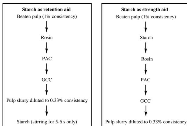
Figure 1 : Sequential addition of chemicals
