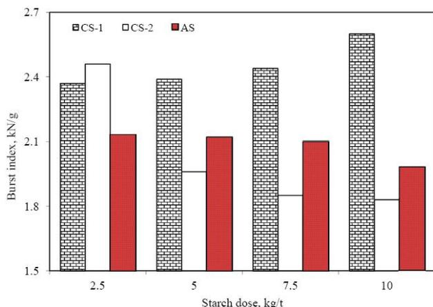
**Figure 4 : Effect of starches on burst index of paper when added in thin pulp stock as retention aid**
