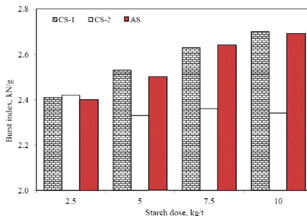
**Figure 9 :** Effect of starches on burst index of paper when added in thick pulp stock as strength aid
