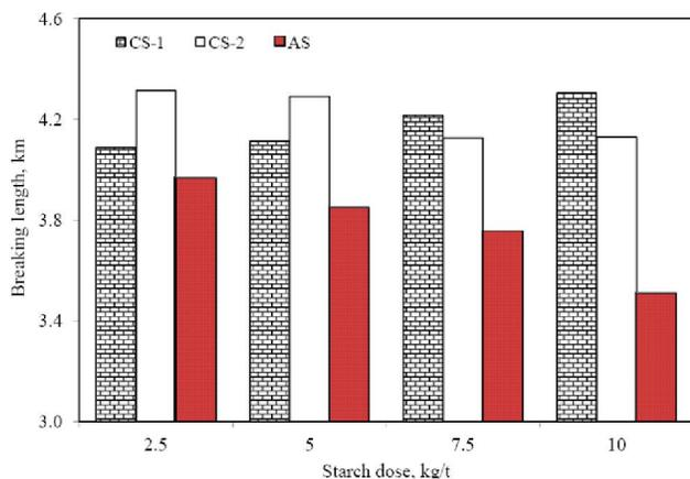
**Figure 8 :** Effect of starches on breaking length of paper when added in thick pulp stock as strength aid
