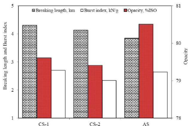
Figure 11 : Paper properties with different starches at 8.5% ash level when used as strength aid
