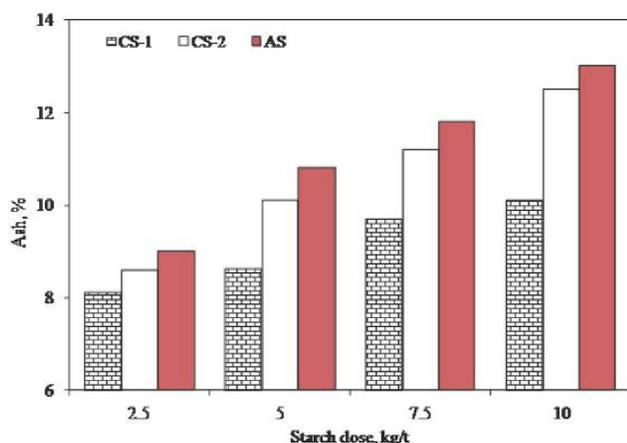
Figure 2 : Effect of starches on ash content of paper when added in thin pulp stock as retention aid
