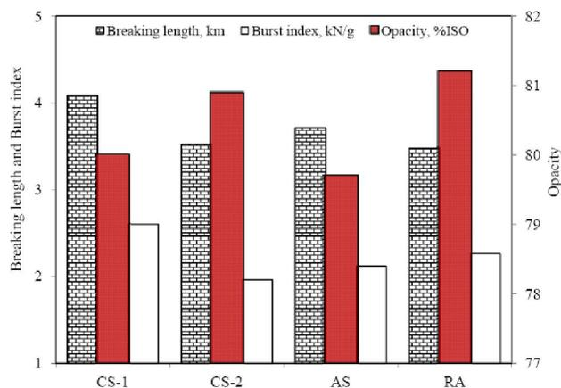
**Figure 6 : Paper properties with different starches and typical retention aid at 10% ash level**
