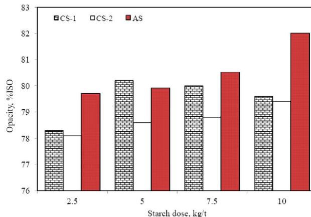
**Figure 10 :** Effect of starches on opacity of paper when added in thick pulp stock as strength aid
