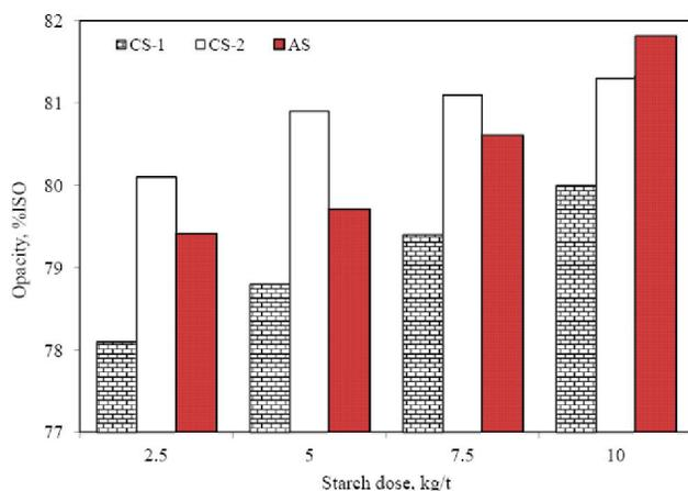
**Figure 5 : Effect of starches on opacity of paper when added in thin pulp stock as retention aid**
