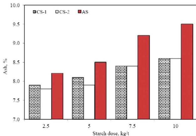
**Figure 7 :** Effect of starches on ash content of paper when added in thick pulp stock as strength aid
