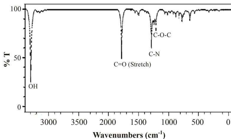
**Fig. 7: Theoretically derived IR spectrum of compound I**
