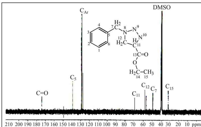
**Fig. 3:**  $^{13}\text{C}$  NMR spectrum of Compound III
