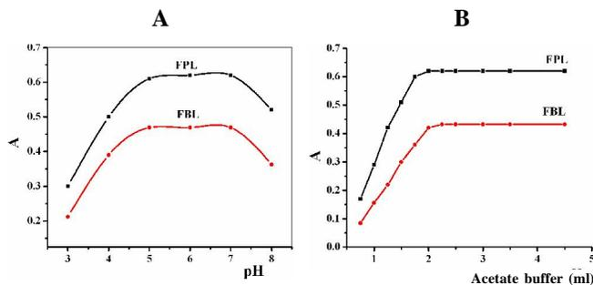
**Figure 2 :** Effect of pH and ml added of acetate buffer on the absorbance of the FPL and FBL complexes in presence of 2.0 ppmMf.
