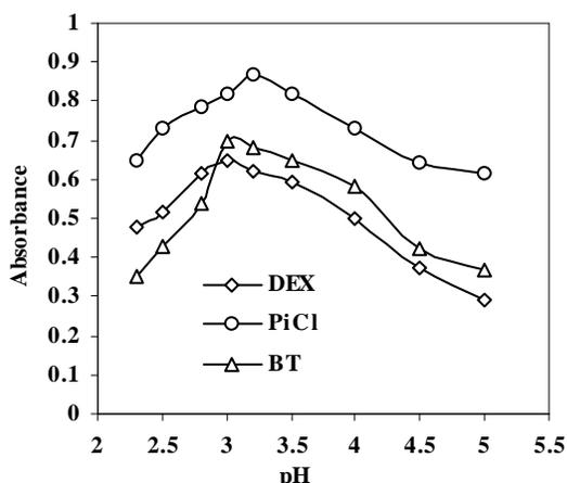
Figure 8: Effect of pH on the absorbance of ( $10 \mu\text{g mL}^{-1}$ ) of the studied drugs with 3 ml of ARS
