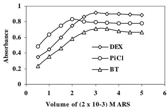
Figure 9: Effect of ARS reagent on the absorbance of the studied drugs ( $10\mu\text{g ml}^{-1}$ )
