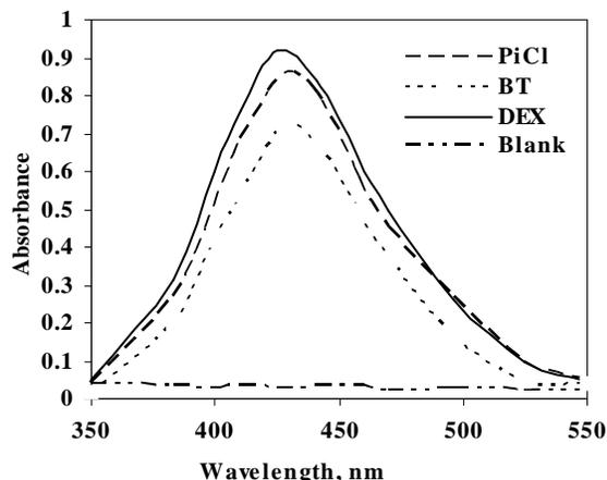
Figure 7: Absorption spectra of ( $10 \mu\text{g mL}^{-1}$ ) of the studied drugs with ( $2 \times 10^{-3} \text{ M}$ ) ARS (.....)
