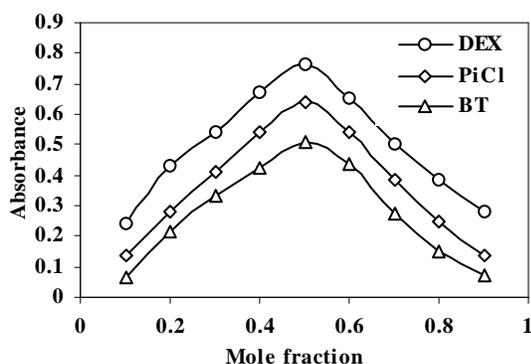
Figure 11: Job's method of continuous variation graph for the reaction of drugs with ARS  $[\text{drug}] = [\text{ARS}] = 1 \times 10^{-3} \text{ M}$
