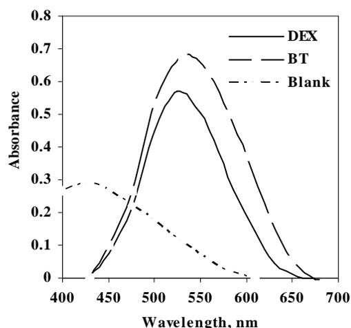
Figure 2: Absorption spectra of reaction products of *p*-CA with  $80\mu\text{g ml}^{-1}$  DEX and  $150\mu\text{g ml}^{-1}$  BT against blank solution.
