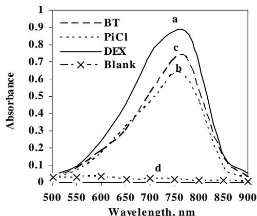
**Figure 4:** Absorption spectra of reaction product between: a- 1 mL of 1 mg mL<sup>-1</sup> DEX and 3 mL of 5 % w/v ammonium vanadate (—), b- 1 mL of 1 mg mL<sup>-1</sup> PiCl and 2 mL of 5 % w/v ammonium vanadate (—), c- 1 mL of 1 mg mL<sup>-1</sup> BT and 2 mL of 5 % w/v ammonium vanadate (—), d- 5 % w/v ammonium vanadate (Reagent blank) (.....)
