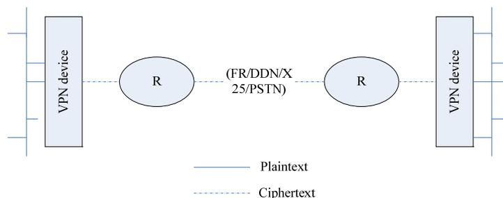
**Figure 2 : Schematic diagram of VPN device configuration**
