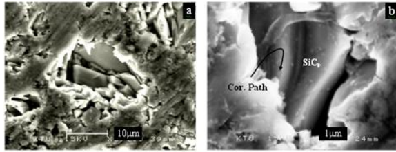
Figure 3: Preferentially corrosion process progressed around SiC particle
