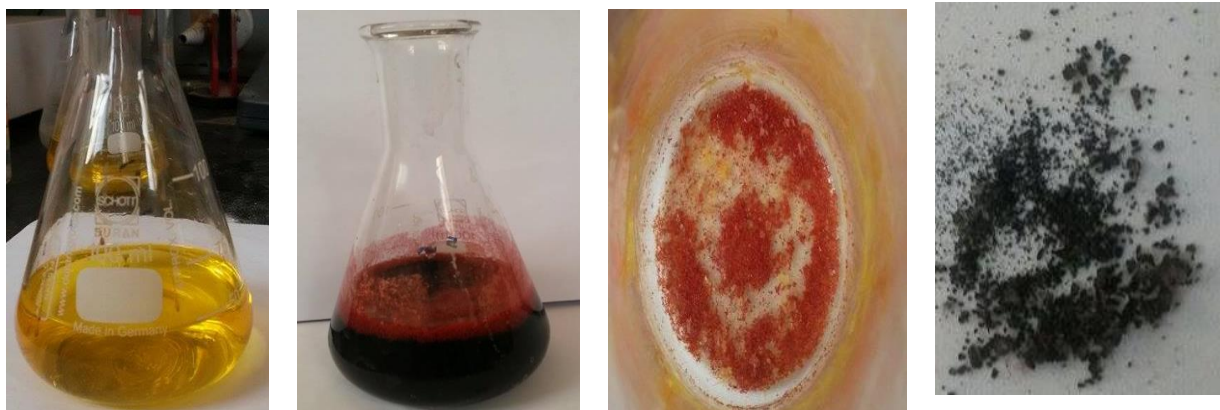
FIG. 8. Successive procedures for vanadium precipitation using ammonium chloride.
