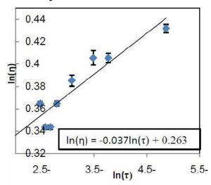
Figure 4 :  $Ln(\eta)$  vs.  $Ln(\tau)$ , using power law  $\eta = \eta'$
