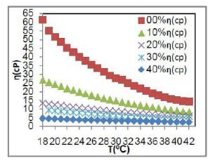
Figure 1: The dynamic viscosity of benzene – coconut oil as a function of temperature at concentrations (00%-40%) by weight of benzene.
