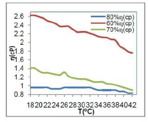
Figure 3 : Dynamic viscosity at different temperatures for 60%, 70%, and 80% by weight of benzene.
