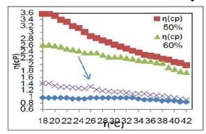
Figure 2 : The dynamic viscosity of benzene – coconut oil as a function of temperature at concentrations (50%-80%) by weight of benzene.
