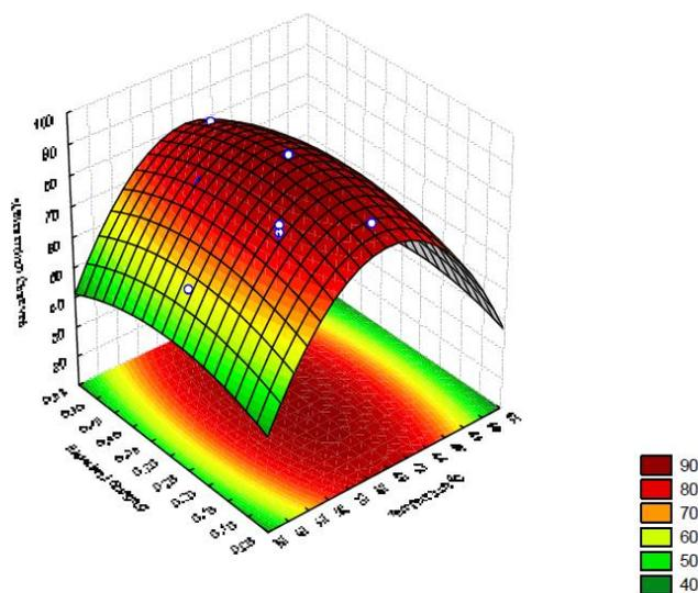
**Figure 3 : Response surface plot of the effects of biosorbent dosage and temperature on percentage biosorption of mercury by *Ficus Hispida* L.**
