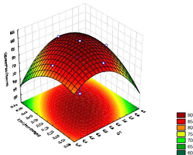
Figure 5 : Response surface plot of the effects of biosorbent dosage and pH on percentage biosorption of mercury by *Ficus Hispida L.*
