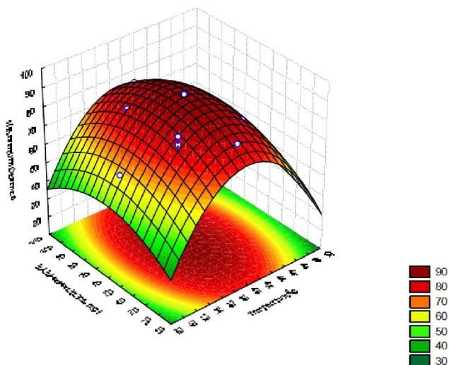
Figure 4 : Response surface plot of the effects of initial metal concentration and temperature on percentage biosorption of mercury by *Ficus Hispida L.*
