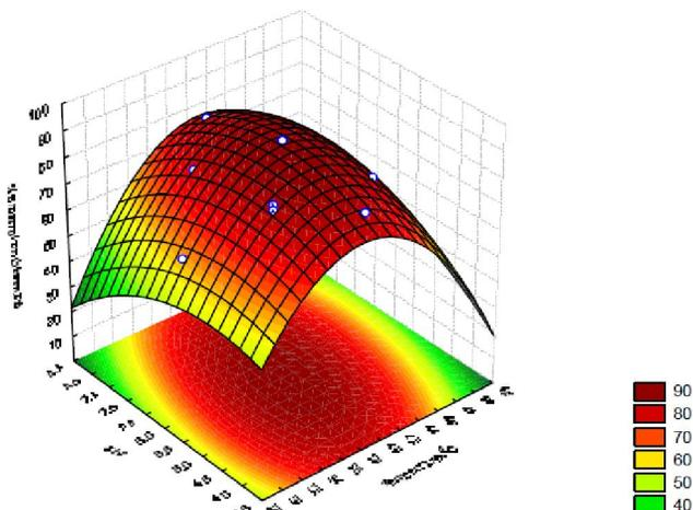
**Figure 2 : Response surface plot of the effects of pH and temperature on percentage biosorption of mercury by *Ficus Hispida* L.**
