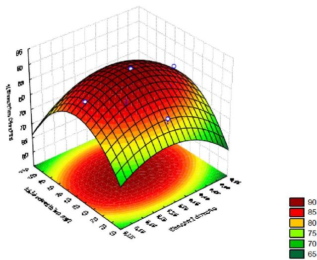
Figure 7 : Response surface plot of the effects of initial metal concentration and biosorbent dosage on percentage biosorption of mercury by *Ficus Hispida L.*
