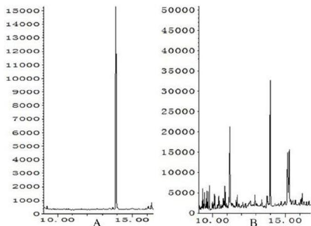
A: the content of standard chlorpyrifos; B: the content of chlorpyrifos in leeks.
