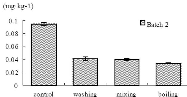
Figure 5 : The concentration of chlorpyrifos during every processing unit operation of batch 2.
