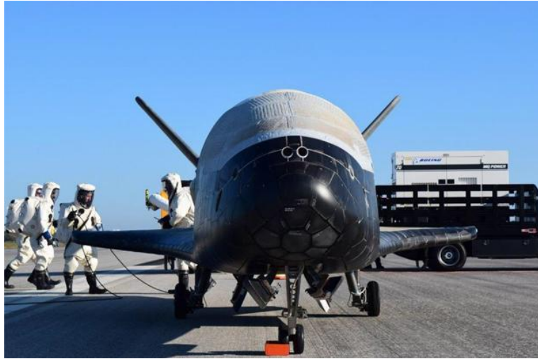
FIG. 5. A view of the X-37B, one of two autonomous military spaceplanes employed on classified missions in low-Earth orbit [39].
