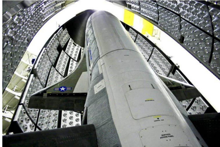
FIG. 2. A launch agreement takes the form of an X-37B spacecraft, encapsulated within a United Launch Alliance Atlas 5 rocket, before the first test flight in April 2010 [24].
