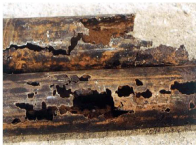
Figure 2 : The tubing corrosion in sour gas reservoirs under existence of bacteria corrosion
