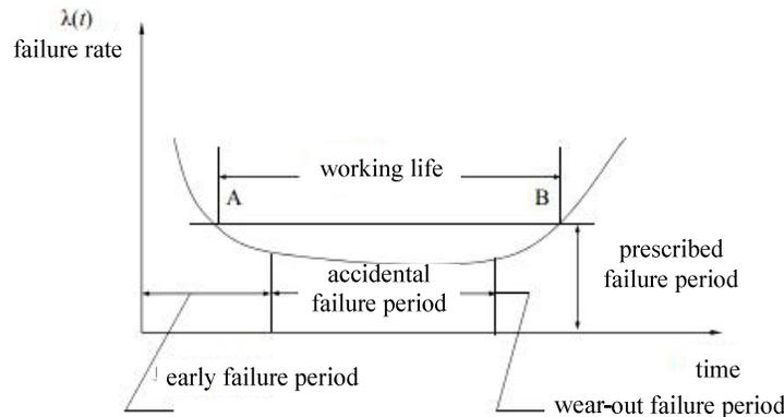
**Figure 2 : Typical failure curve (bathtub curve)**
