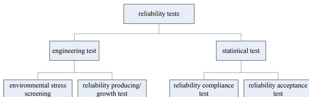
Figure 1 : The classification of common reliability tests
