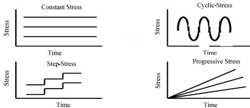
Figure 3 : Types of the life accelerating testing
