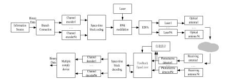
Figure 1: System model of space optical communication based on MIMO Optical MIMO channel model
