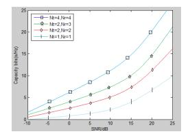
Figure 2: Curves of channel capacity and SNR
