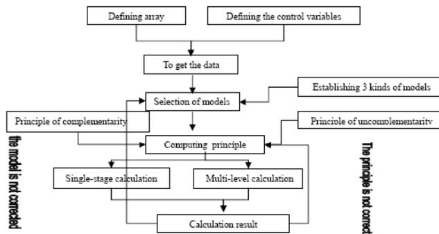
**Figure 1 : Calculation flow chart on catastrophe progression model**
