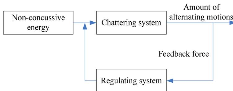
Figure 1 : The constitution of the self-excited chattering system
