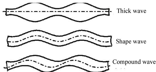
**Figure 5 : The geometric characteristics of chattering wave**
