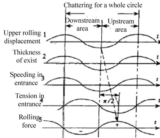
Figure 2 : The forming process of self-excited chattering
