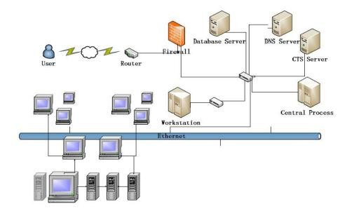
Figure 5: The network structure of agricultural product supply chain management system
