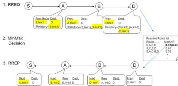
Figure 6 : Routing tables by extend AODV
