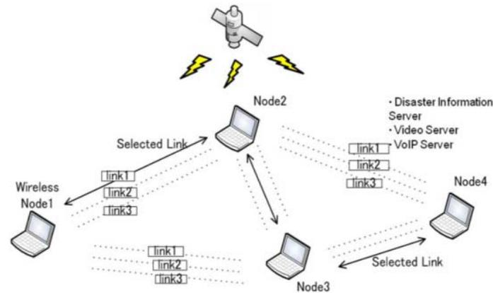
**Figure 4 : Wireless network architecture**
