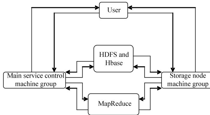
**Figure 3 : Storage structure of the large amount of data**
