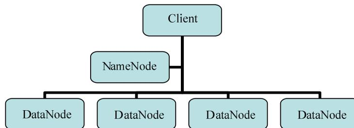
**Figure 2 : Simplified diagram of hadoop**
