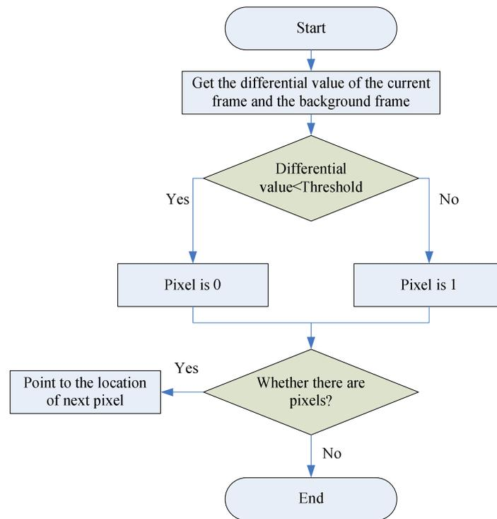
Figure 2 : The flowchart of background subtraction
