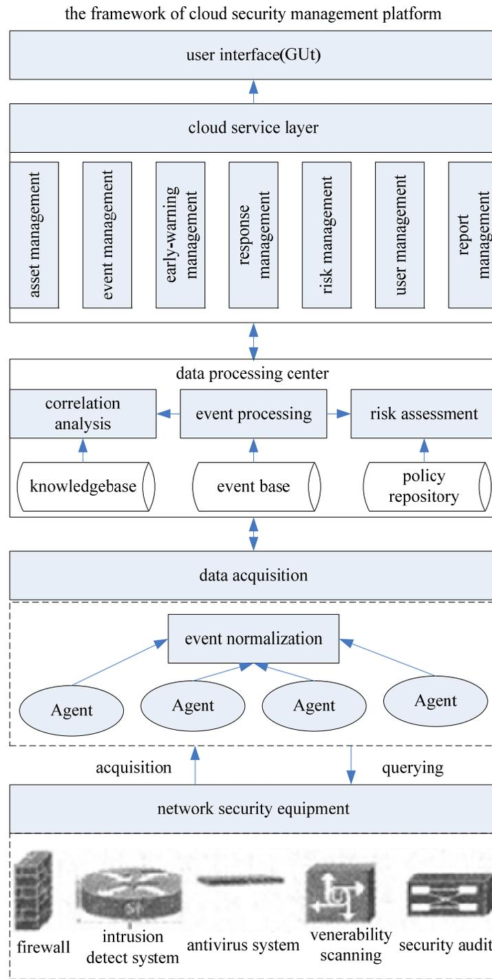
**Figure 3 : The framework of cloud security management platform**
