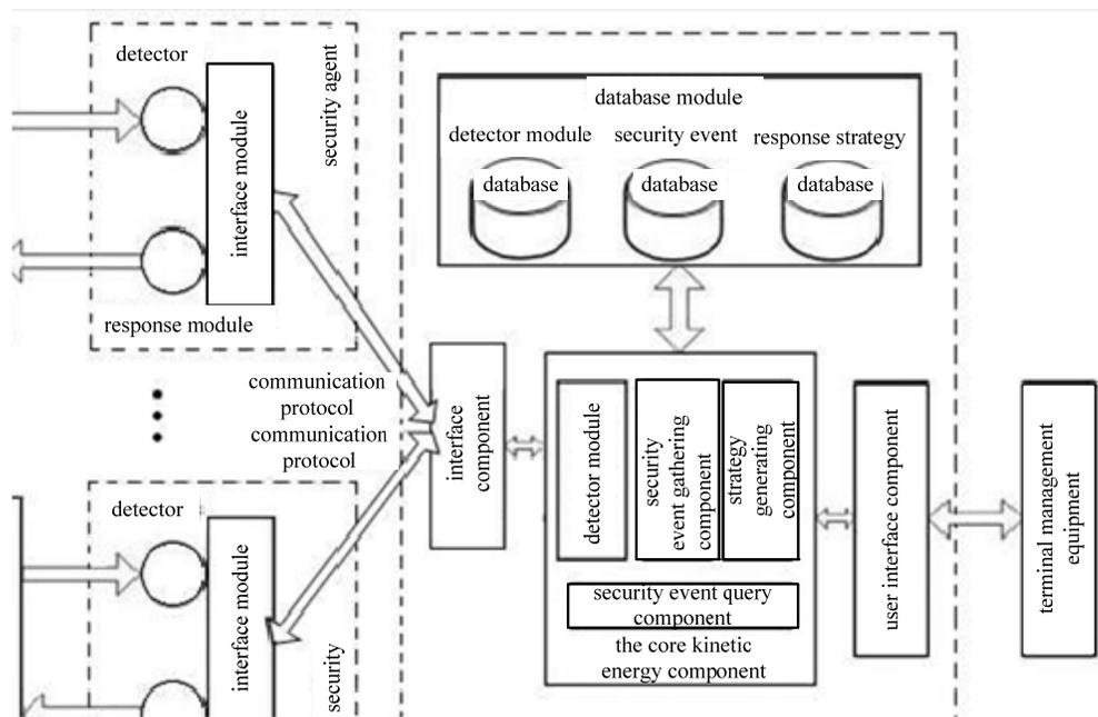
**Figure 4 : Schematic diagram of enterprise’s security management system structure**
