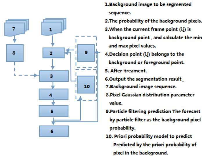
Figure 1 : Algorithm overall flow chart
