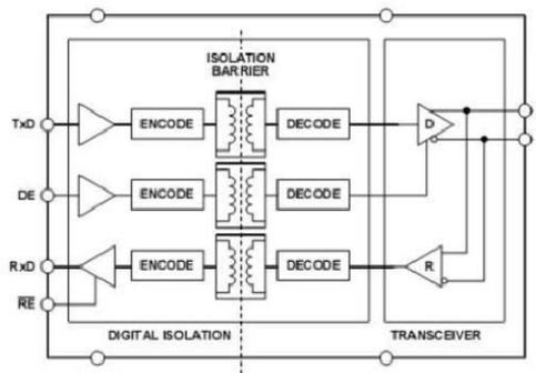
Figure 2: Schematic of internal serial communication
