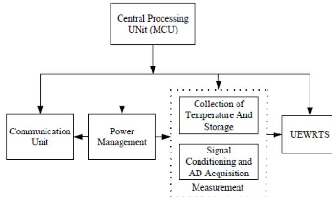
Figure 1: Block diagram of collector
