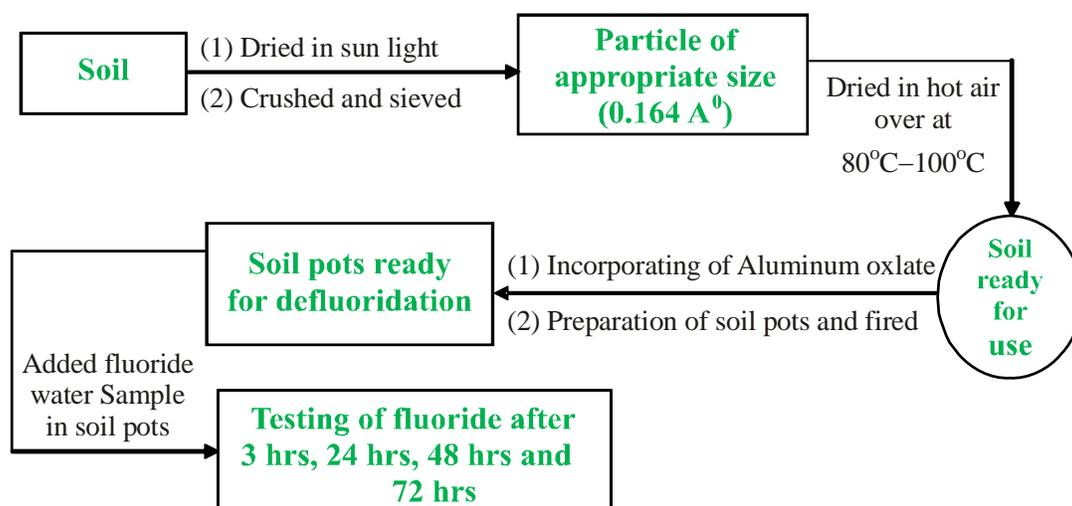
Fig. 11: Flow chart of adsorbent (soil pots) preparation and fluoride adsorption on to soil pots
