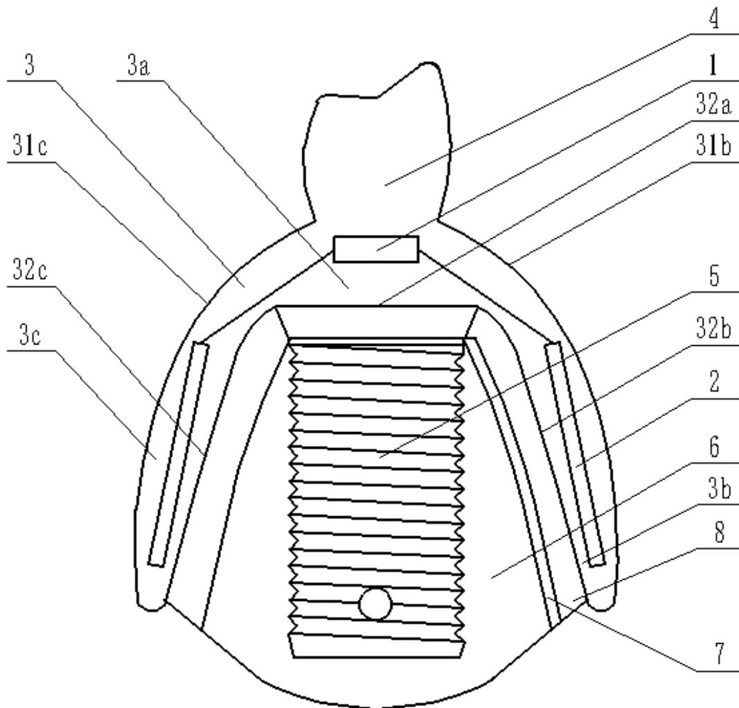
1-Power supply; 2- electrode plates; 3- denture base;3a- the top of the denture base; 3b- buccal denture base; 3c- lingual denture base; 31b- the polished surface of buccal denture base; 31c - the polished surface of lingual denture base; 32a- the top surface of denture soft tissue; 32b- buccal tissue surface of the denture base; 32c- lingual tissue surface of the denture base; 4- dentures; 5- implants; 6- cancellous bone; 7- cortical bone; 8- gingival mucosa
