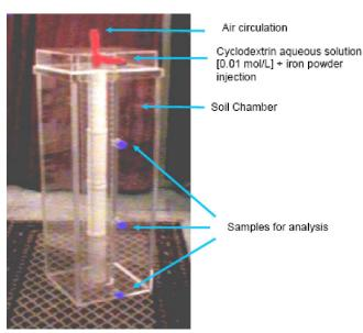
Figure 1: Prototype soil column treatment using  $\beta$ -cyclodextrin, detergents and zero valent iron. Column external dimensions are 30 cm x 30 cm x 150 cm; and internal dimensions are 10 cm x 10 cm x 150 cm. This compartment is perforated from the bottom to the top. Sampling heights from the top of the column for analysis are: 5 cm, 55 cm, and 110 cm.
