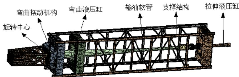
Figure 2: Structure model of fatigue testing machine
