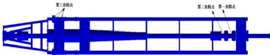
Figure 3: Three dangerous points of fatigue testing machine by static analysis
