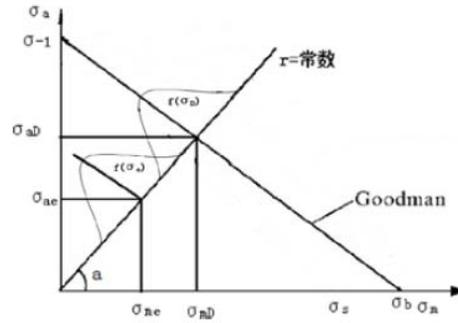
**Figure 1: Equal life curve and stress- strength interference relationship**
