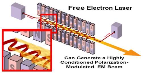
Figure 8 : Precise, highly modulatable electromagnetic beam formed by electron beam passing through dipole magnets.
