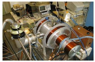
Figure 13 : Chamber with a Helicon RF plasma generating system at the Australian National University
