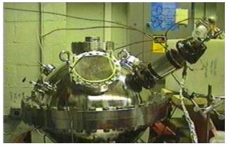
Figure 6 : Ion gun embodied in IEC reactor at University of Illinois
