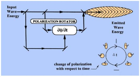
Figure 2 : Generation of polarization-modulated EM radiation
