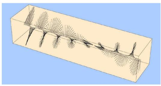
Figure 3 : Rapid change in E field configuration during 1 polarization-modulation cycle by an SU(2) beam.
