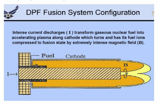
Figure 11 : Dense plasma focus fusion propulsion for flight
