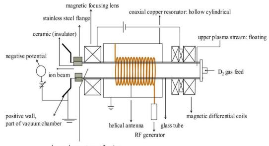
lower plasma stream: floating Figure 7 : Elements embodied in one of the ion guns used in the University of Illinois IEC reactor
