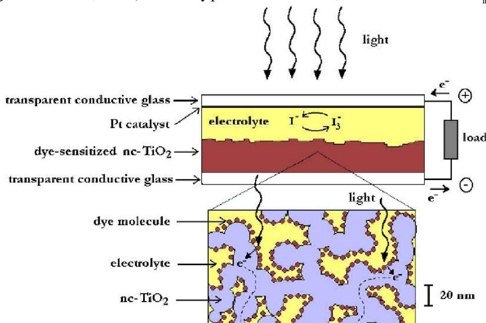
Figure 1 : Schematic representation of dye sensitized solar cell
