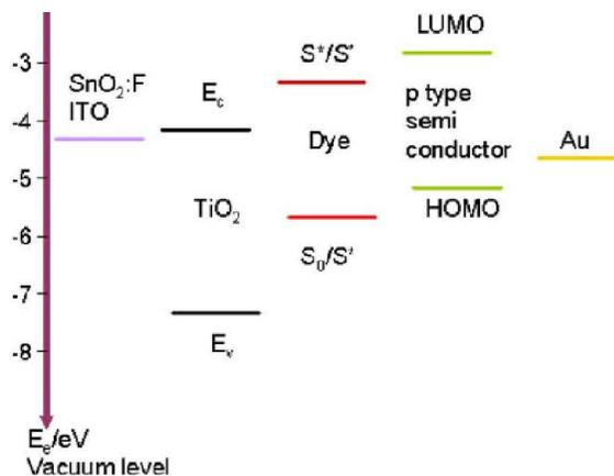
**Figure 5 : Energy diagram for an efficient charge transfer between solid state dye sensitized solar cell components**
