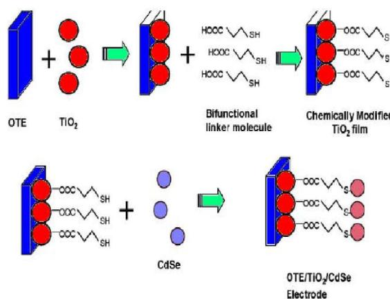
**Figure 6 : Linking CdSe QDs to TiO<sub>2</sub> surface with a bifunctional surface modifier**
