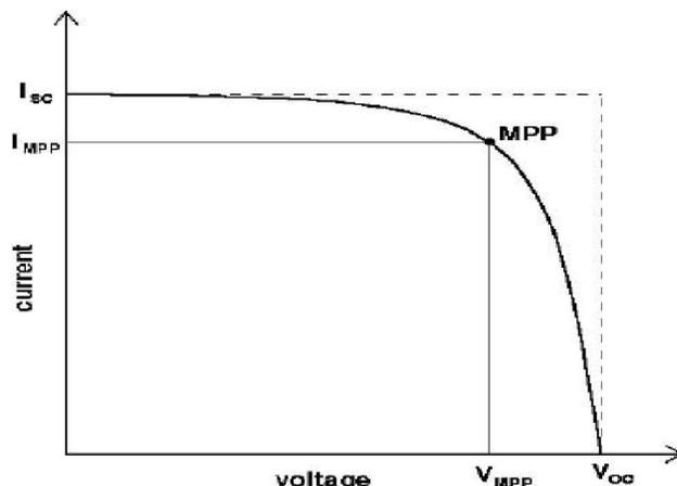
**Figure 3 : Current–voltage (I-V) curve of an organic solar cell**
