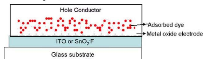
Figure 4 : Schematic description of a solid state dye sensitized solar cell
