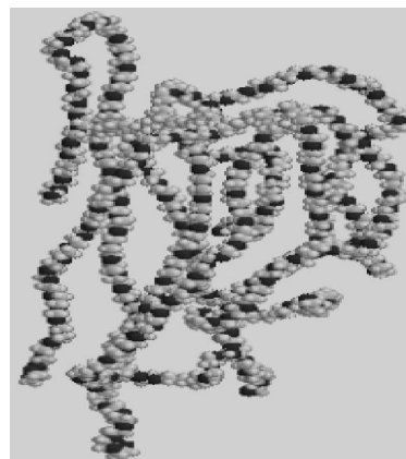
Figure 1 : Molecular structure of an amphiphilic polymer having (black) hydrophilic and (white) hydrophobic parts
